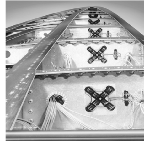
Complex stresses developed within this airplane wing are analyzed from strain gauge data.
