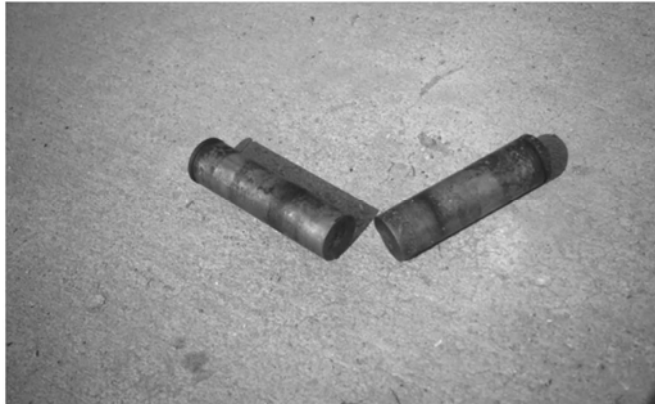
The pin was made from a hardened steel alloy, that is, one having a high carbon content. It failed due to brittle fracture.
